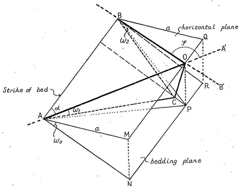
Fig. 9 Determination of strike and dip of a bed.
