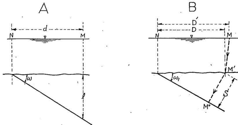
Fig. 10 CSP's record (A) and actual profile (B)
