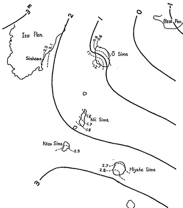
Fig. 11 Geoid contours around the Izu Islands in the SAO-SE3 system, extended from the astrogeodetic geoid map of Japan by Ganeko (1976).
