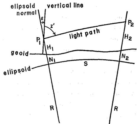
Fig. 3 Geometry of trigonometric levelling. Ellipsoidal height  $h = H + N$
