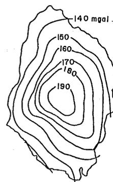
Fig. 9 Free-air gravity anomaly over Ō Sima.
