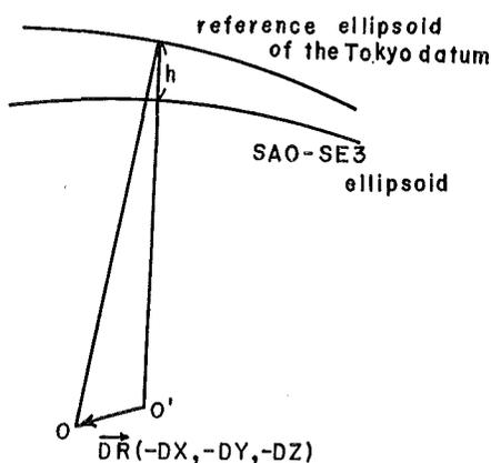
Fig. 8 Conversion of geodetic datums.
