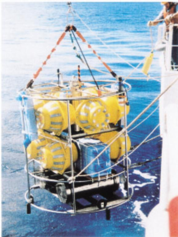
Fig. 3 Photo of SeaFAR (one of twin unit) just before the placement on the sea floor in 1997 at Southern East Pacific Rise.
