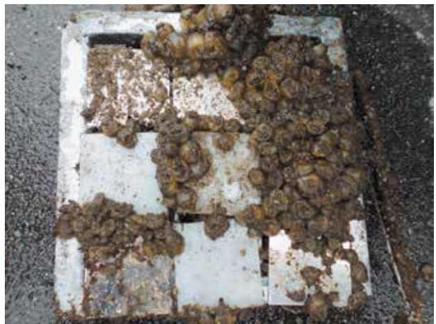
Photo 5. Results of antifouling tests. See Table 3 for antifouling paints used.
