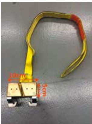
Photo 3. Recovery device for the AOV. 写真3. 回収用治具.
