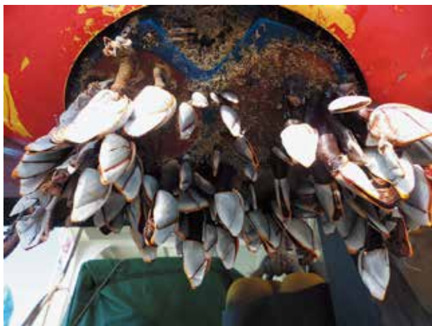
Photo 4. (a) Solar panel of the AOV covered with seaweed. (b) Shellfish on ADCP.
