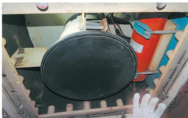
Photo 1. The transmission part of the newly installed multi-acoustic ranging system.
