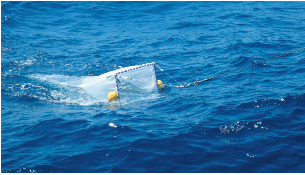
Photo 9. Neuston net being towed in such position that the seawater enters through the opening of the net.
