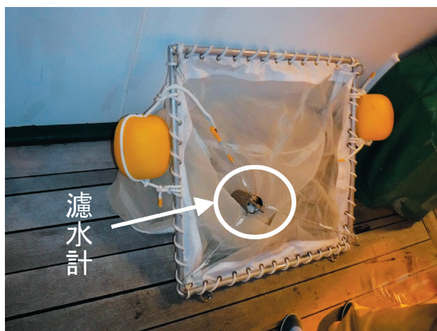
Photo 5. Attaching a flow meter to the neuston net. 写真5. 濾水計の取り付け。
