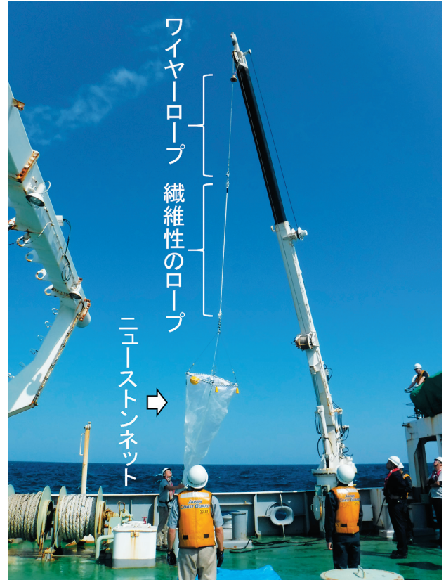
Photo 7. Connecting the crane and the neuston net. Fiber rope connects the crane cable and the net.
