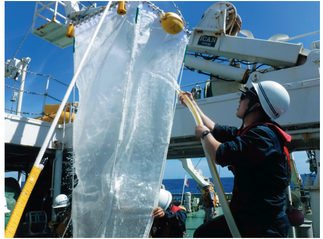
Photo 10. Washing the neuston net. Water is applied from the outside to collect all samples in the cod end.
