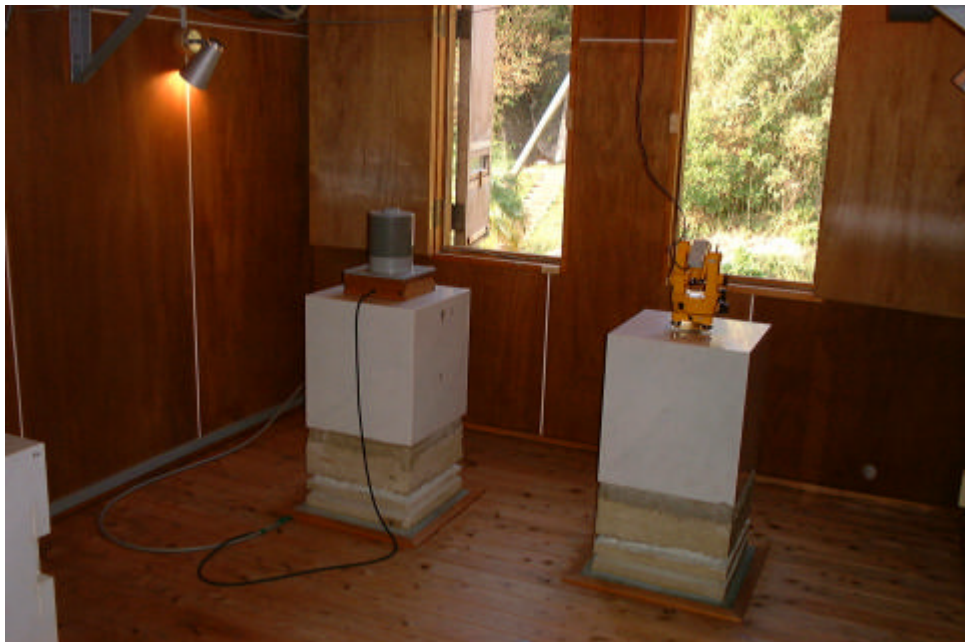
Magnetometer mounted on the Instrument Piers of Absolute Observation House
