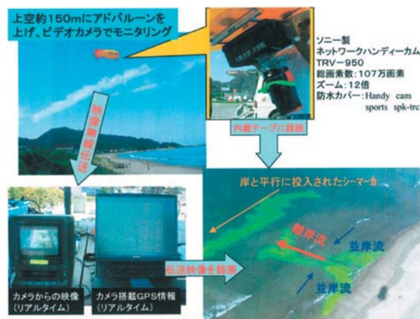
Fig.E 2 Observation system using balloon with video camera (upper panel) and sea-marker (lower right panel) (Furukawa and Yamashiro, 2003).
