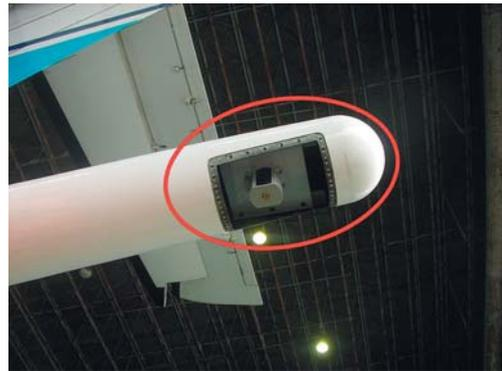
Photo. 4 The detector installed in the tail stinger.
