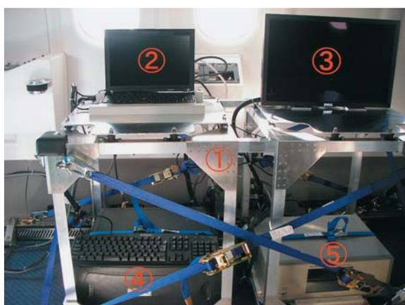
Photo. 7 Equipments attached in the rack (①: Rack with equipment, ②: Airplane position indication equipment, ③: Magnetic data indicator, ④: Infrared camera data collection container, ⑤: Magnetic data collection container).
