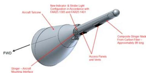
Fig. 1 The structure of the tail stinger (non-magnetism).
