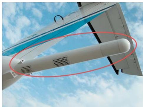
Photo. 3 The tail stinger attached to after most part of MA 725.
