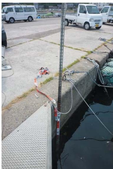
Photo. 3 Simultaneous tidal observation (sensor lifting).
