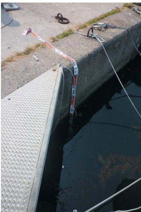
Photo. 2 Simultaneous tidal observation (sensor lowering).
