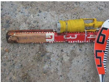
Photo. 1 Sensor attached to a tide pole.
