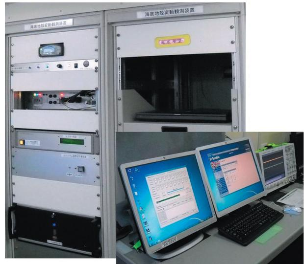
Photo 1 Recording device of seafloor geodetic observation system installed on the S/V “Kaiyo.”
