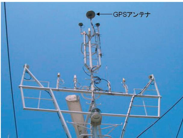
Photo 3 Installation of a GPS antenna at the mast of the S/V “Kaiyo.”
