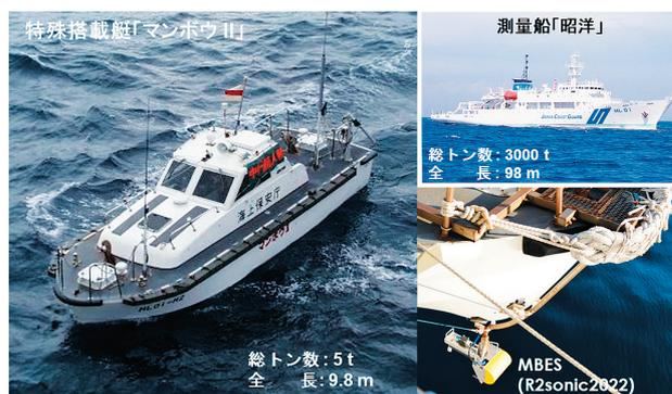
Photo 2. Autonomous survey boat *Manbo II* (left), her mother vessel, S/V *Shoyo* (upper right), and an MBES (R2sonic2022) mounted on the *Manbo II* (lower right).
