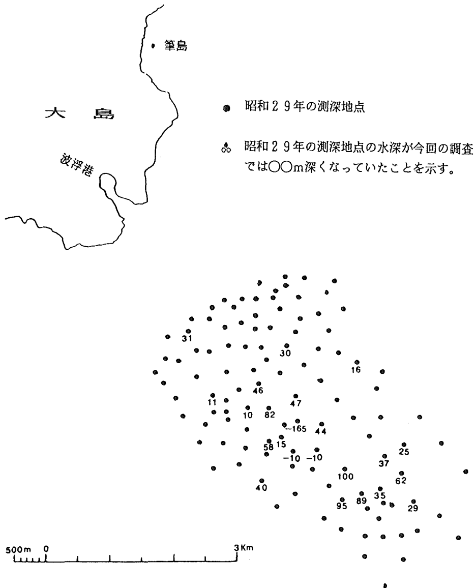
Figure 7 Sounding points in 1954 and depth changing (more than 10m) points from 1954 to 1987
