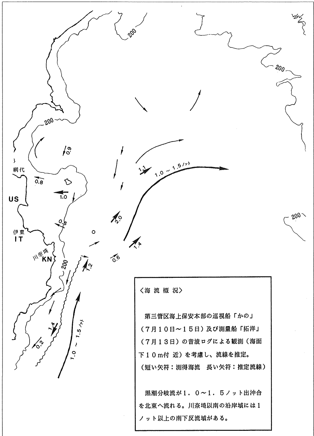
Figure 18. Current at the sea east of Izu Peninsula, deduced from observed data by Acoustic Doppler Current Plofiler of patrol vessel "Kano" and survey vessel "Takuyo" during July 10 to 15, 1989.
