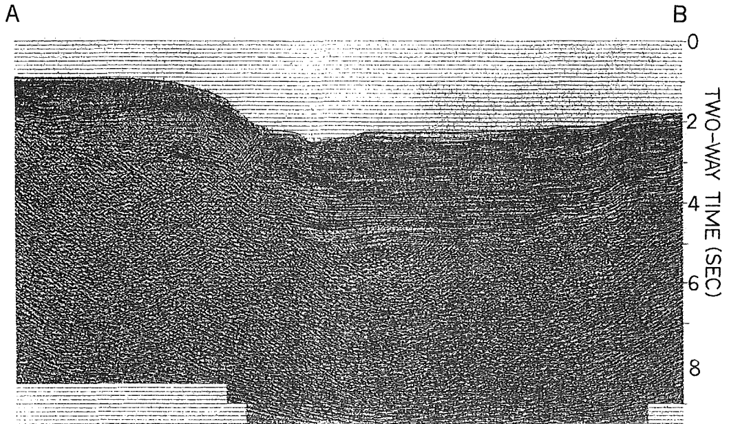
Figure 7-a. The multi-channel seismic profile migrated in time domain between A and B on the line No. 17 in figure 6.
