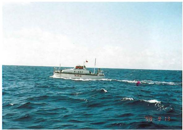
Photo 4. Intelligent survey boat "Manbou II" sounding Myozin Syo submarine volcano
