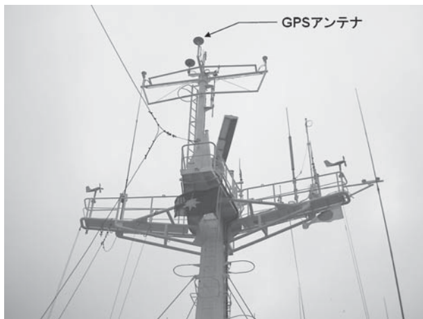
Photo. 3 Installation of the antenna on the mast for GPS observation.
