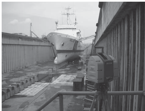
Photo. 5 Measurement by leveling method for calculating the position relation between the devices.
