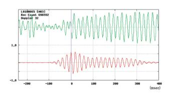
Fig. 4 Received signal (upper) and the result of cross-correlation (lower).
