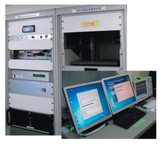
Photo 1 Recording device of seafloor geodetic observation system installed on the S/V "*Kaiyo*."
