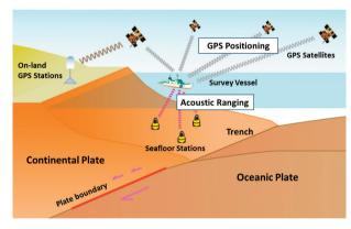
Fig. 1 Schematic picture of seafloor geodetic observation.
