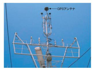
Photo 3 Installation of a GPS antenna at the mast of the S/V "*Kaiyo*."
