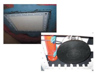
Photo 2 Installation of an acoustic transducer on the bottom of the S/V "*Kaiyo*."
