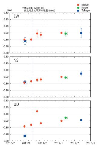
Fig. 7 Time series of the estimated positions at the seafloor reference point "Sagami-wan" from December 2010 to September 2012. Each marker shows observation by the S/V "Meiyo" (red), the S/V "Kaiyo" (green) and the S/V "Takuyo" (blue).
