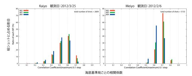
Fig. 5 Comparison of correlation coefficient calculated from acoustic ranging data measured by the S/V "Kaiyo" (left) and the S/V "Meiyo" (right). M02, M03 and M04 show the identification codes of the seafloor stations.
