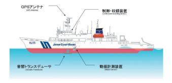
Fig. 2 Situation of installation of GPS/acoustic seafloor geodetic observation system on the S/V "Kaiyo."
