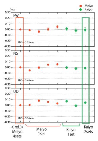
Fig. 6 Comparison of the positioning results by the S/V "Meiyo" (left) and the S/V "Kaiyo" (right) relative to the result using all data of "Meiyo" at "Sagami–wan." See text for detail.
