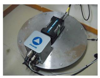
Photo 4 Installation of a motion sensor, PHotonic Inertial Navigation System (PHINS).
