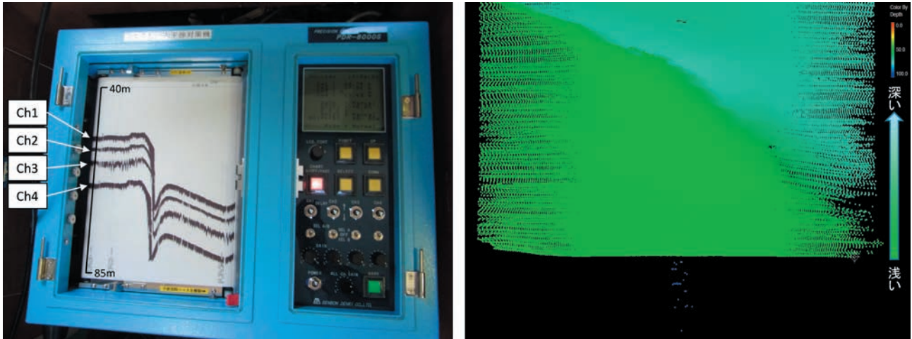
Photo 4. PDR-8000SDZ records at lowered transmit power of ‘+1’ (left) and Sonic2024DH sounding data (right) in depth of approximately 50–70 m. Even if transmit power of PDR-8000SDZ is reduced, record quality is sufficient at the depth of at least approximately 70 m. In addition, few interference noises appear in the sounding data of Sonic2024DH.
