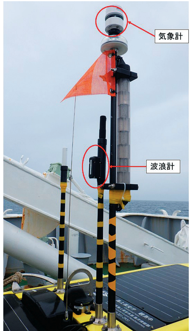
Photo 10. Weather station and wave meter on AOV. 写真 10. AOV の気象計と波浪計。
