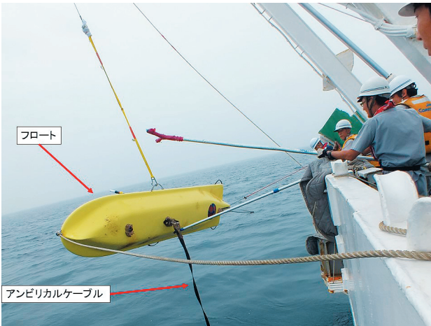
Photo 4. Lifting the AOV's float.
