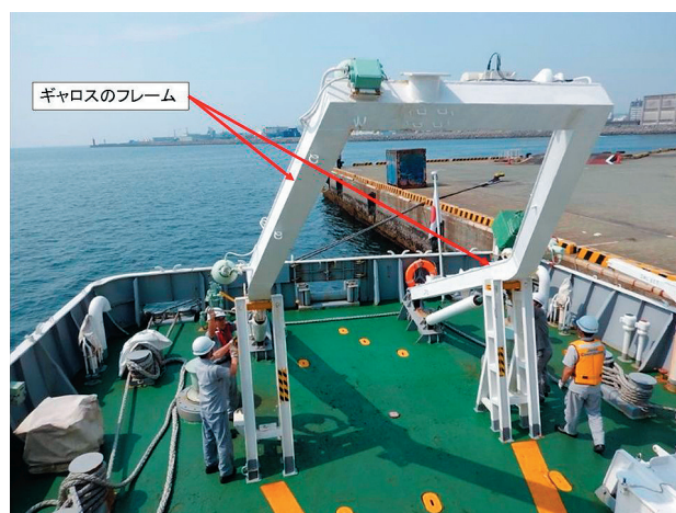
Photo 2. [S/V Meiyo] Recovery workspace. These particular types have frames on both side of the A-frame crane.
