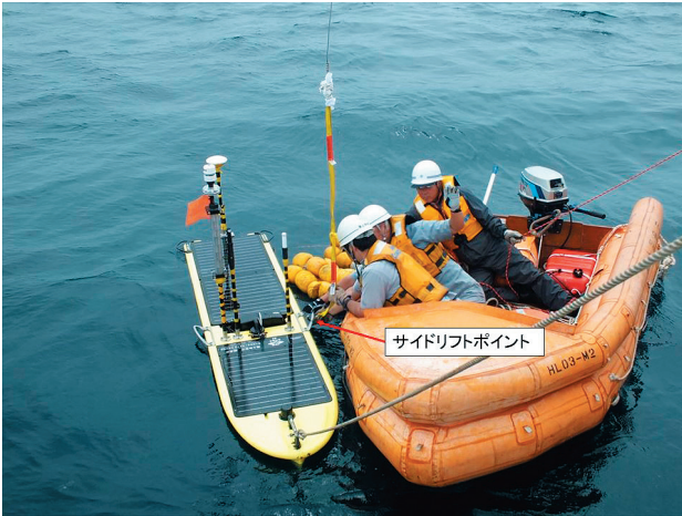
Photo 3. Attaching lifting rope to the side lift point of the AOV.
