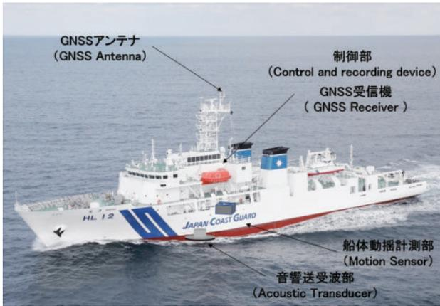
Photo 1. Positions of installed equipment for the GNSS-Acoustic observation on the S/V *Koyo*.
