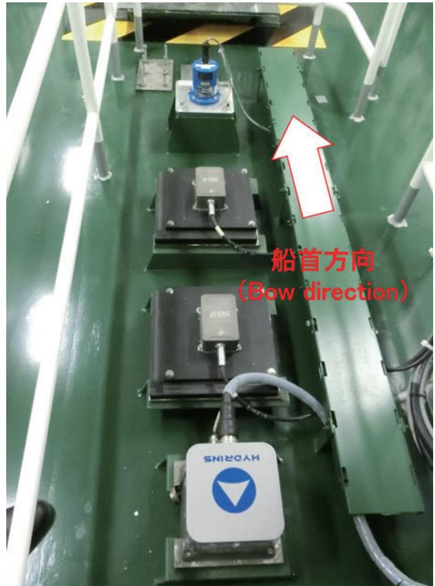
Photo 3. Dynamic motion sensor "HYDRINS" (the innermost one).
