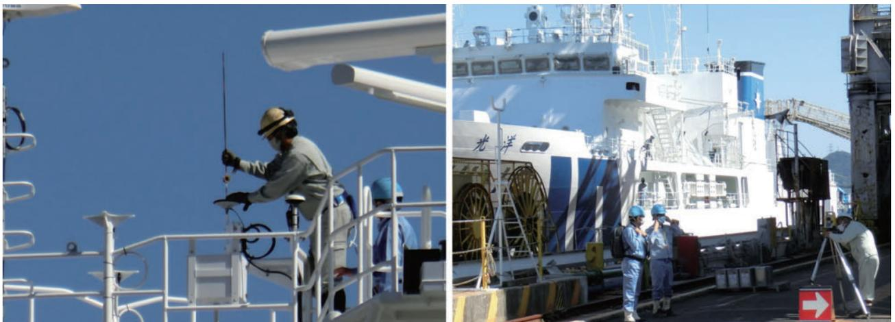
Photo 7. Survey for relative positioning of the GNSS antenna to the acoustic transducer using a total station.
