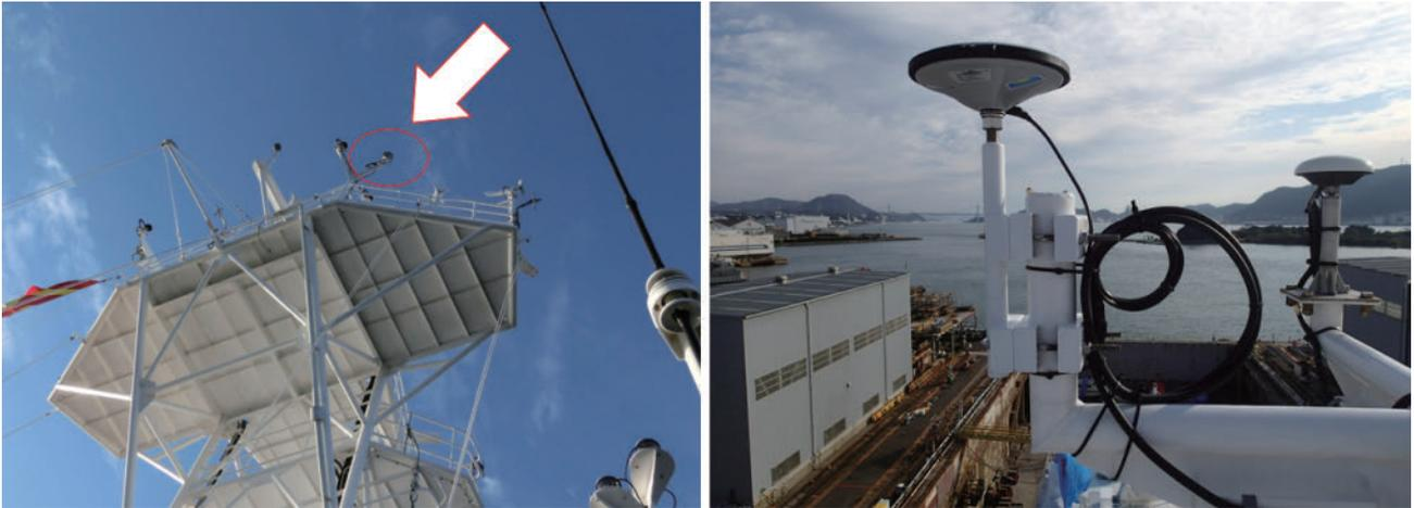
Photo 5. GNSS antenna installed on the mast of the S/V Koyo.
