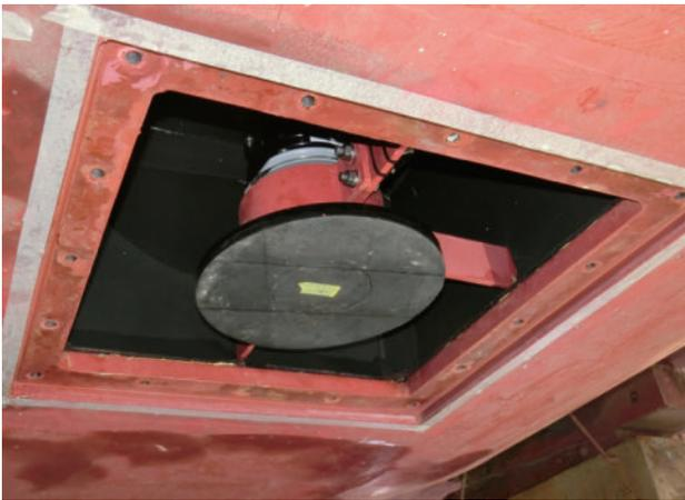
Photo 2. Acoustic transducer to be mounted on the hull of the S/V *Koyo*.
