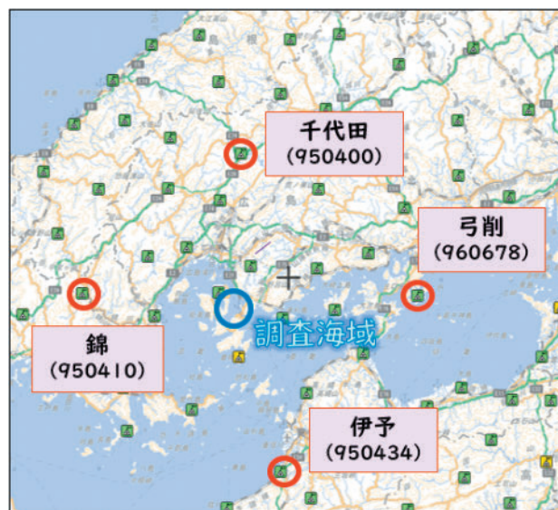
Fig. 10. Used GNSS CORSs: a spatially balanced array of four base stations at longer distances from the survey area.
