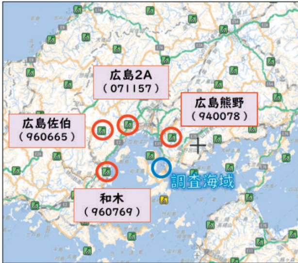
Fig. 11. Used GNSS CORSs: an unbalanced array of four base stations at adequate distances from the survey area.
