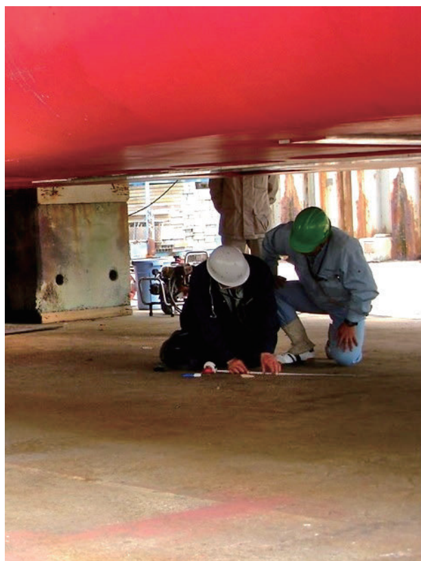
Photo 1. Marking on the dock floor below the transducer reference point for S/V Meiyo .
