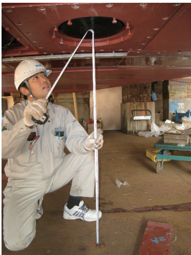
Photo 3. Height measurement between the dock floor marker and the center of transducer plane for S/V Takuyo in 2010.
