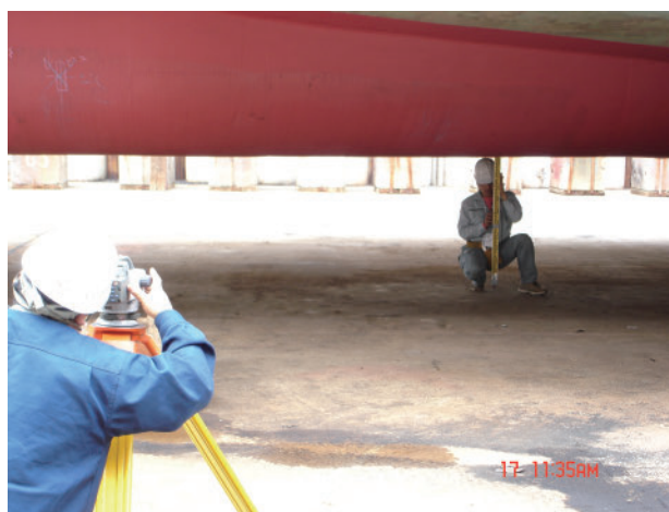
Photo 2. Leveling between the dock floor marker and the center of transducer plane for S/V Meiyo . Adopted from Kawai et al. (2009).
