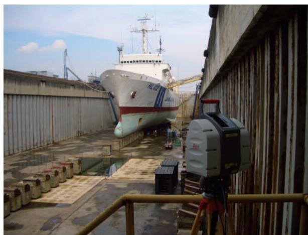
Photo 4. Angle and distance measurement for S/V Takuyo in 2014.
