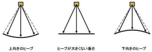
Fig. 3. Schematic of soundings when the vessel undergoes heave motion near the surface sound speed gradient.
